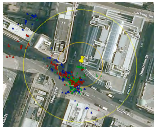
Figure 4: The first 10 min positioning solution for test 1
