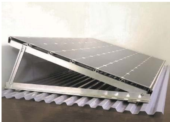
Figure 6: Modified sub-construction based on a Tritec mounting system for corrugated metal roofs. The sub-construction is adapted to the mounting of a SUC-module with rear side aluminum beams. In this example a frameless glass/backsheet with 0.8 mm glass thickness has been applied.
