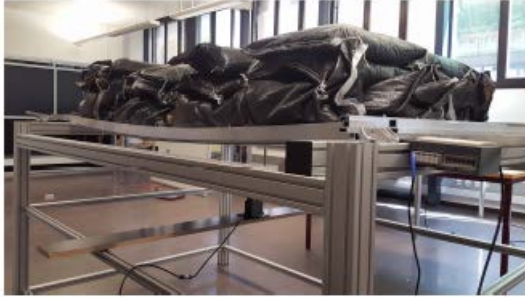
Figure 3: Laminate with applied mechanical load in form of sandbags on the back side of the laminate.
