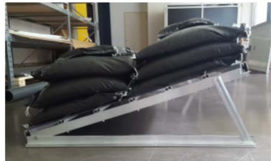
Figure 5: PV laminate and sub-construction under load demonstrating the mechanical stability of the construction.
