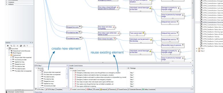
SAHRA allows to capture STPA Step 1 and 2 analysis in the visual style of mind map diagrams. The analysis information is captured by individual elements reflecting for example Keywords, UCAs, Hazards, and Losses. This provides maximum flexibility to the analyst in terms of documenting the analysis. Drag and drop from the lower left panel allows to easily create new elements. Drag and drop from the lower right panel allows to reuse existing elements while inheriting existing relationships.
