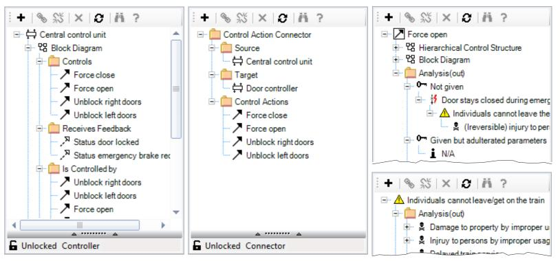
SAHRA's context sensitive object browser shows information for the currently selected element: controller (left), control action connector (center), control action (top right), hazard (bottom right).
