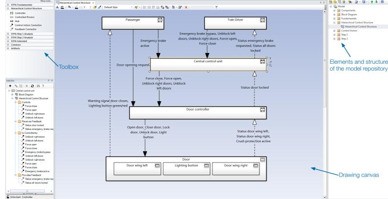
Screenshot of SAHRA as extension for the UML/SysML tool Enterprise Architect. The model of a Hierarchical Control Structure is shown in the center of the screenshot. The controller 'Central control unit' is currently selected. The toolbox (top left) contains all elements needed for capturing STPA diagrams. The model repository and its structure is shown in the repository tree (right).
