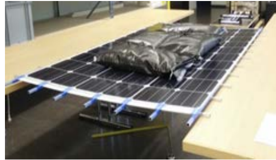
Figure 2: Laminate with applied mechanical load in form of sandbags on top.
