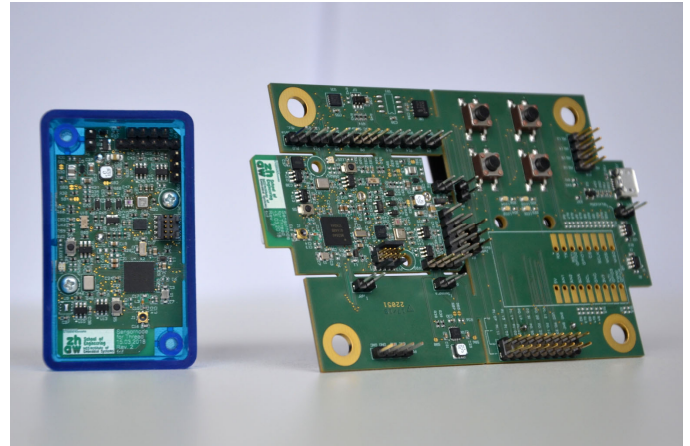
Fig. 8. Hardware implementation of Leaf Node
