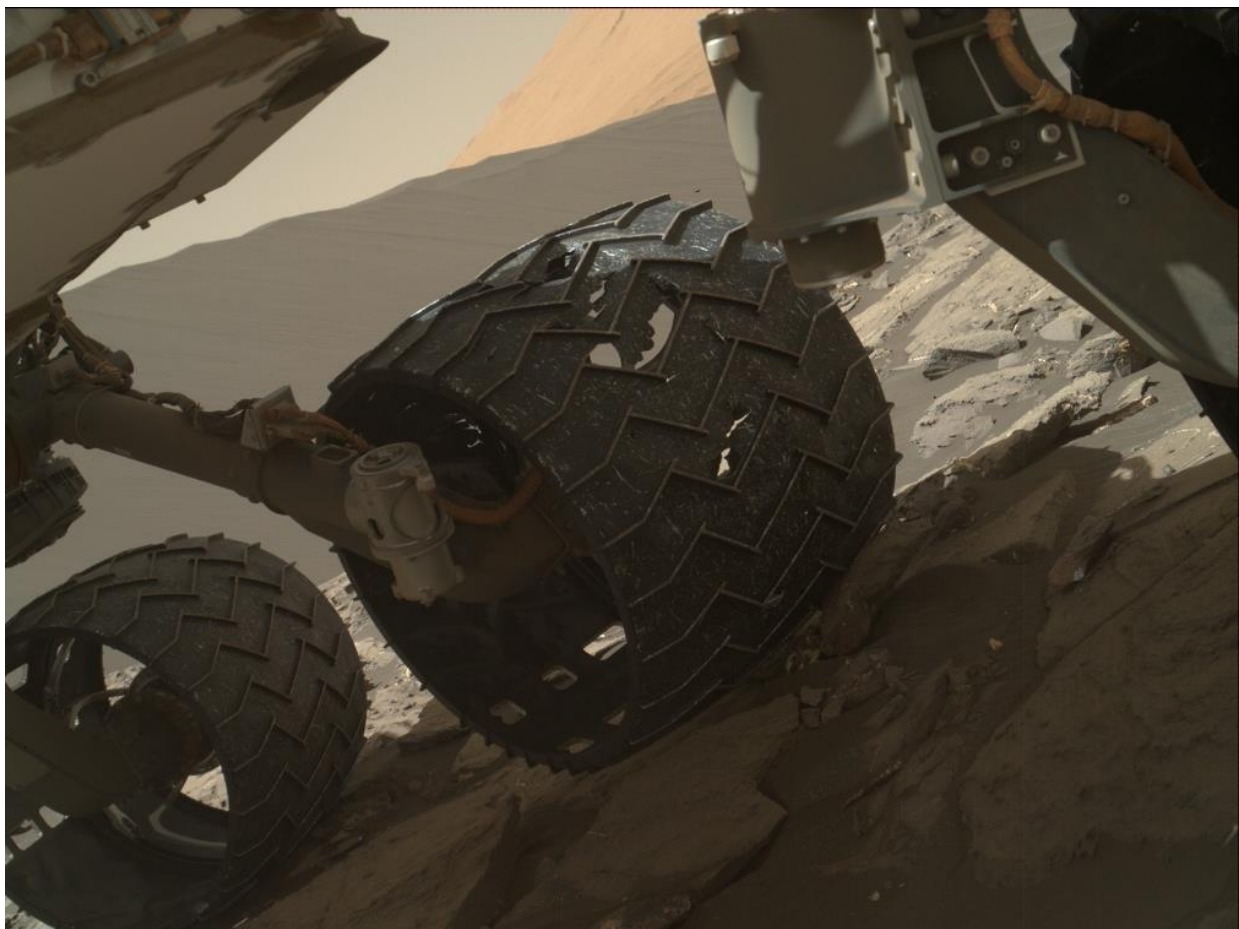
Figure 56: Wheel Damage on MSL 127
