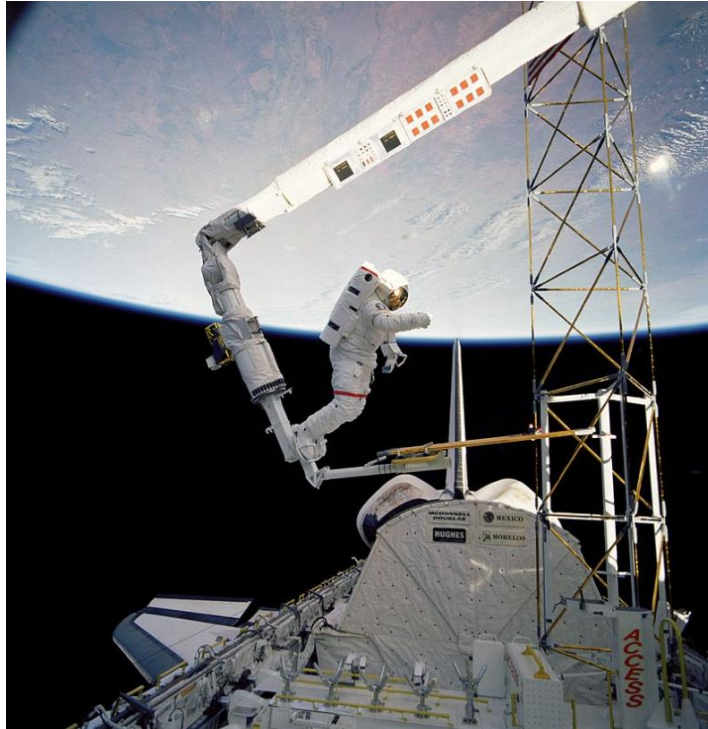
Figure 31: Assembly of the ACCESS Experiment during STS-61B 79
