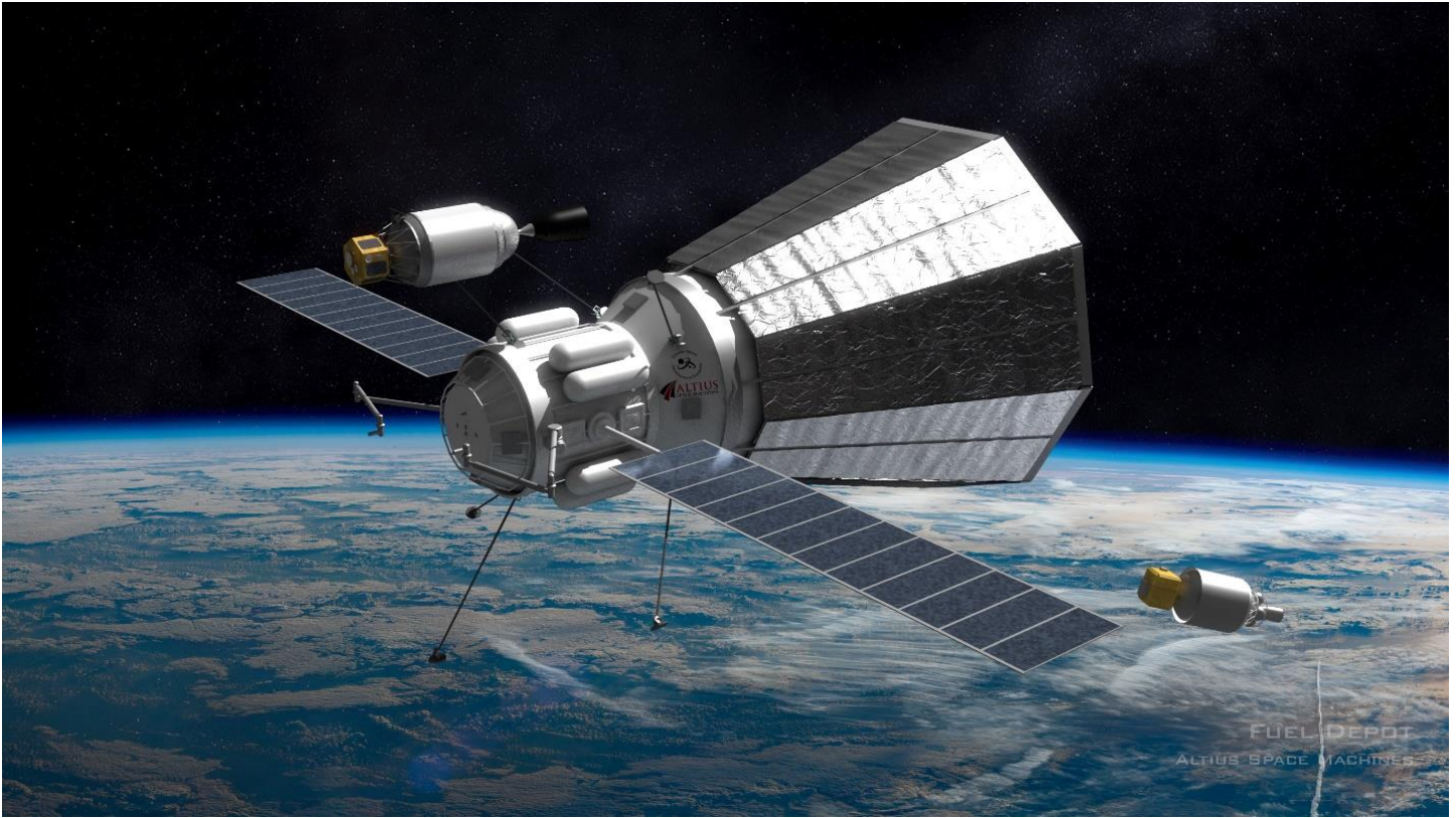
Figure 39: Artist's Conception of a LEO Propellant Depot for Smallsat Launch Vehicles Shown using EMBARC boom-assisted magnetic capture technology for direct rendezvous/capture of smallsat launch vehicle upper stages
