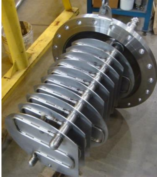
Figure 19: Ice Collection Plates of a Commercial CT Operated by Paragon to manage water in their vacuum test facilities.
