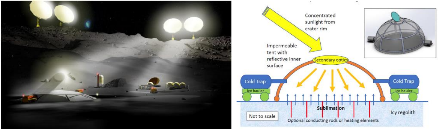
Figure 26: Conceptual Power System Using Heliostats at a Moon Crater
