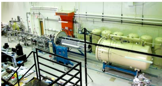
Figure 1. The 3 MV dust accelerator installed in the CCLDAS Lunar Environment and Impact Laboratory. The accelerator is used to simulate the effects of dust impacts with speeds \gg 10 km/s for micron sized projectiles. The facility will be also used to test and calibrate plasma and dust instruments, including the Lunar Dust Experiment (LDEX) for the LADEE mission. The facility is now operational and available for the lunar community for impact studies.
