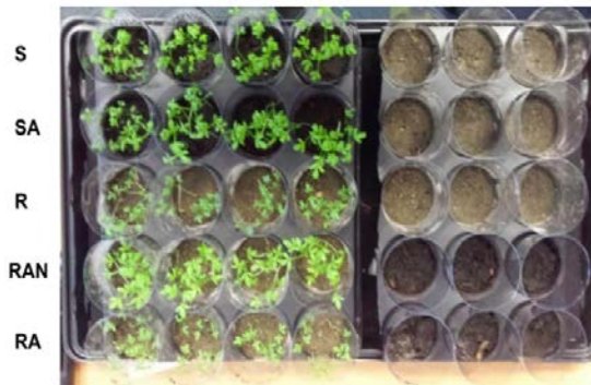
Figure 1: Experimental setup for plant growth analysis on regolith simulant Eifel soil. Left side with rows of cress: RA - autoclaved regolith, RAN - autoclaved regolith with nutrients, R - regolith, SA - autoclaved peat, S - peat. On the right side soil samples without plants to analyze contamination effects during watering and cultivation period. Regolith soil differs in color comparing to the dark peat
