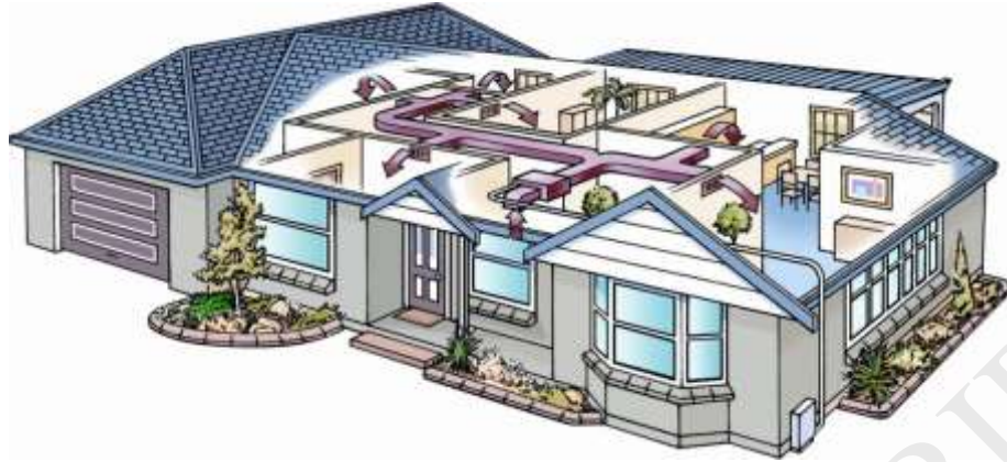
Fig. 17. Ducted air systems [80]
