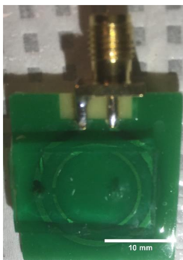
Figure 4-12 Picture of a PDMS-channel sensor.
