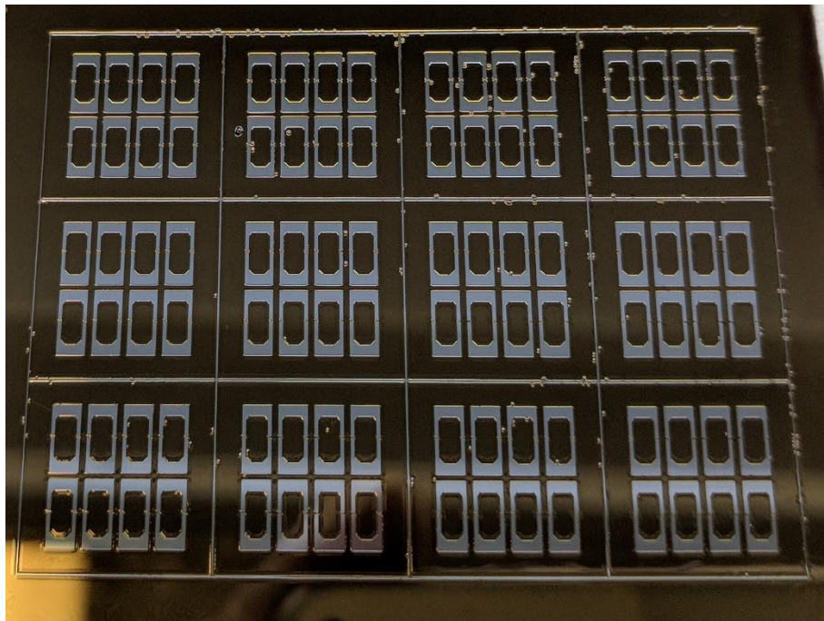
Fig. 4.2: A photo of the sample backside after development.
