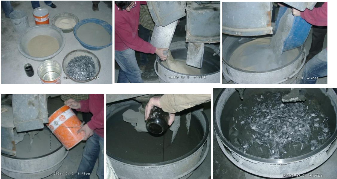
Figure 3. Mixing process of steel fibers concrete
