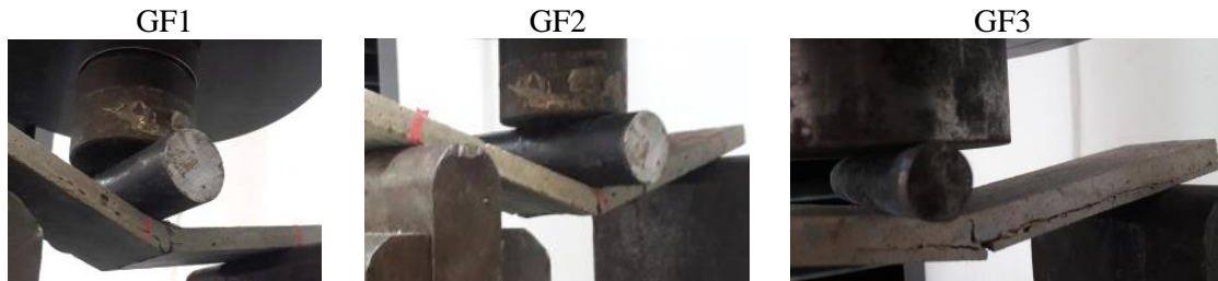
Figure 9. Views of cracked samples from test setup
