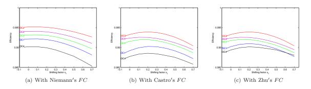
Fig. 16: Efficiency values when Niemann's, Castro's and Zhu's friction coefficients were implemented (third case study)
