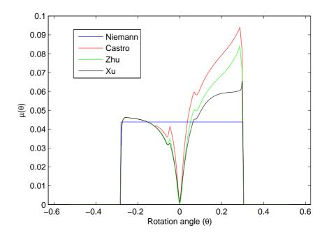
Fig. 1: Friction coefficient formulations example (159 Nm and 1500 rpm)
