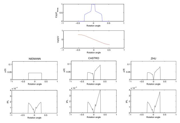
Fig. 4: Comparison among factors, on which efficiency depends, for the three FC formulations (159 Nm and 1500 rpm)
