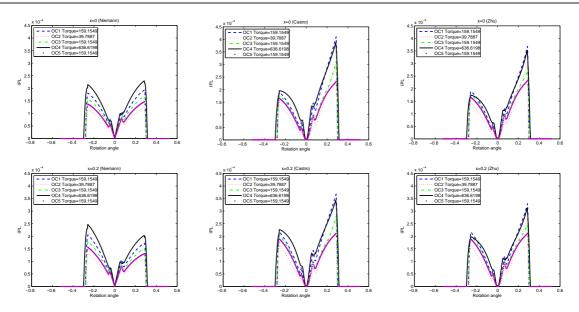
Fig. 10: *IPL* factors, when three *FC*s were implemented, in the extreme cases of profile shifting  $(x_1 = 0 \text{ and } x_1 = 0.2)$
