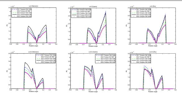
Fig. 15: *IPL* factors, when the three *FC*s were implemented, in the extreme cases of profile shifting  $(x_1 = 0 \text{ and } x_1 = 0.5)$
