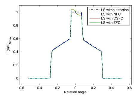
Fig. 3: Load Sharing formulations: example with no shifting profile (159 Nm and 1500 rpm), when no friction coefficient is implemented, with Niemann's (NFC), with Castro's (CSFC) and with Zhu's (ZFC) friction coefficients
