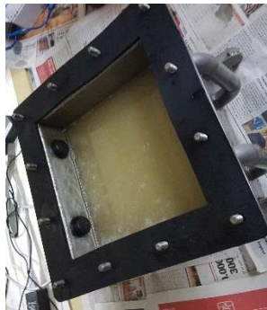
(a) Transformer tank
