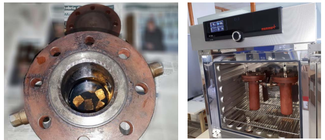
Fig. 5. (a) Test pieces in the vessel filled with dielectric oil; (b) Vessels containing the oil-impregnated samples being introduced in the convective oven to start the ageing process.
