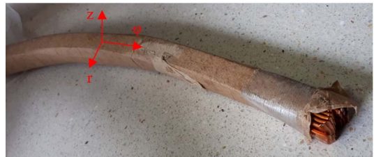
Fig. 2. Real CTC conductor which will be analysed in the laboratory with its cylindrical coordinate system.
