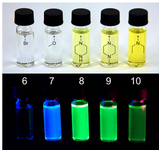
Fig. 1 Monomers 6–10 in solution (DMSO) under visible light ( top ) and UV irradiation ( \lambda = 365 nm)
