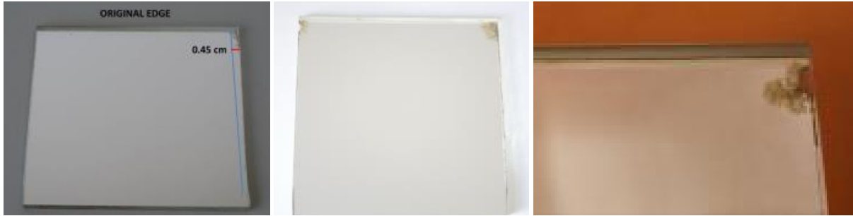
FIGURE 3. Degradation at the non-protected edges of samples tested by #2 (left), #3 (center) and #5 (right) after the NSS test.
