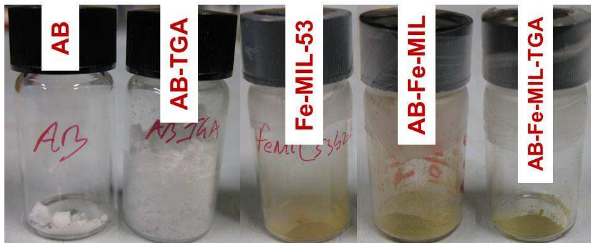
Figure S6. Photographs of pristine AB and Fe-MIL-53, and AB-Fe-MIL (1:1 AB:Fe) samples before and after thermal dehydrogenation (TGA) shows the extensive sample foaming is suppressed in nanoconfined AB sample.
