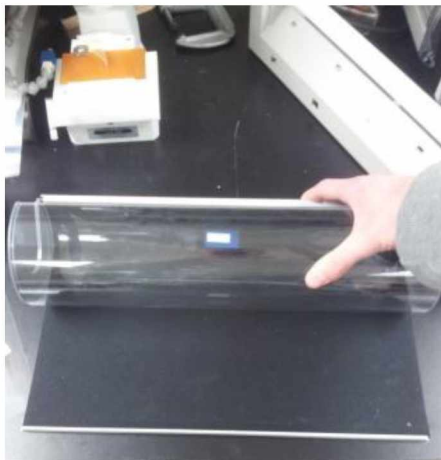
Figure 67: SR-3000 and channel pattern being wrapped in the Letralite blanket before being placed over the black light.
