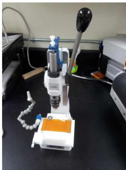
Figure 16: Schmidt Press MHPM-UNV with 0.023 inch Hole Punch (Schmidt Technology Corp., PA).
