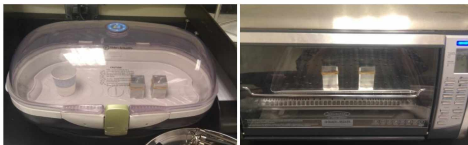
Figure 30: Samples in vacuum desiccator for degassing and oven for curing.
