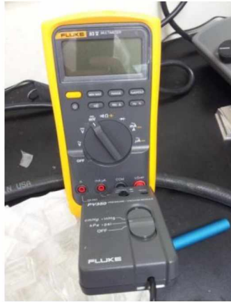
Figure 24: Teqequipment Net (NJ) Fluke pressure transducer module and multi-meter.
