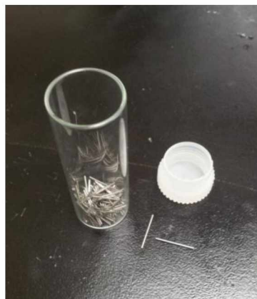
Figure 26: Itronix Inc. (CA) rounded tip stainless steel probes.
