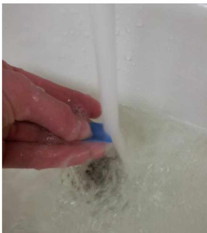
Figure 32: 3mm x 3mm SR-3000 being washed with warm water for 1 minute and 30 seconds.
