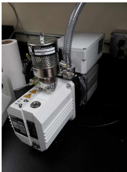
Figure 18: Oerlikon Corp. (Switzerland) Trivac D2,5E vacuum pump.
