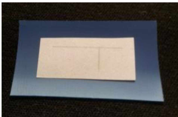
Figure 66: SR-3000 film rough matte side up underneath the Letralite black light with the printed side of the UV vellum against the rough side of the SR-3000.
