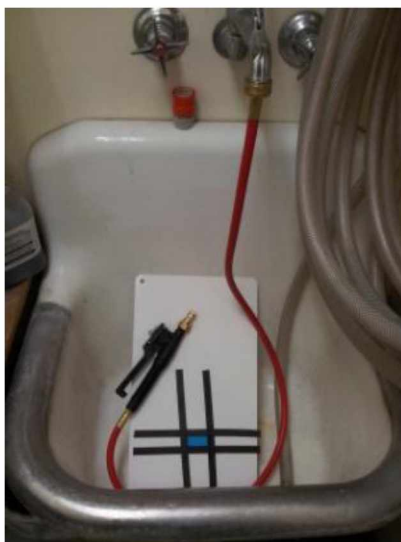
Figure 68: SR-3000 sheet prepared for washout.
