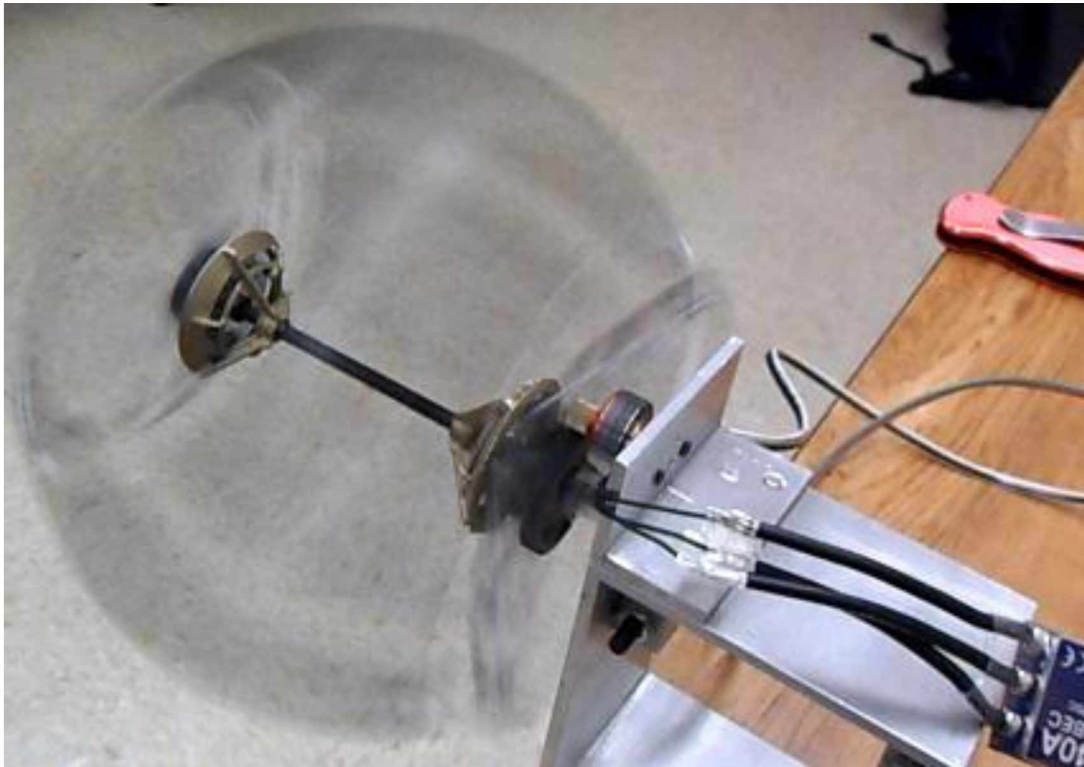
Figure 28: Spinning cycloidal rotor to perform force and power testing.
