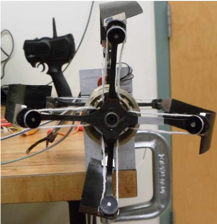
Figure 27: Demonstrating the pitching of the airfoils to the designed \pm 40^\circ .
