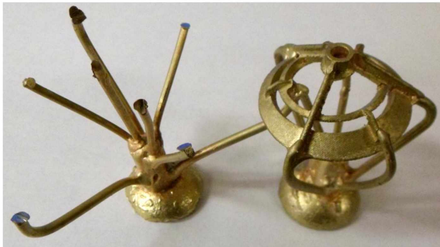
Figure 22: Sprue tree with lost wax casting bronze pitching mechanism.
