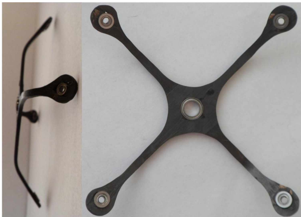
Figure 24: Carbon fiber spider supports with bearings inserted.
