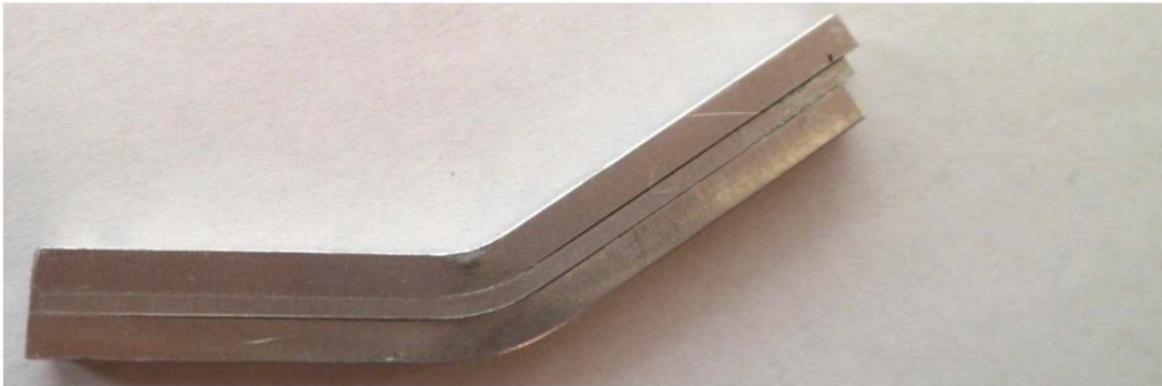
Figure 21: Test specimen of two 3.175 mm heat treated aluminum with 1.5875 mm in the middle where the carbon fiber arms will be determining the differential length needed in the arms.
