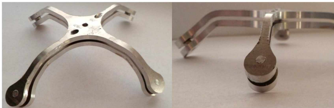
Figure 19: Compression molds shown with pegs and center location hole as well as an angled hole for pulley support drilling.
