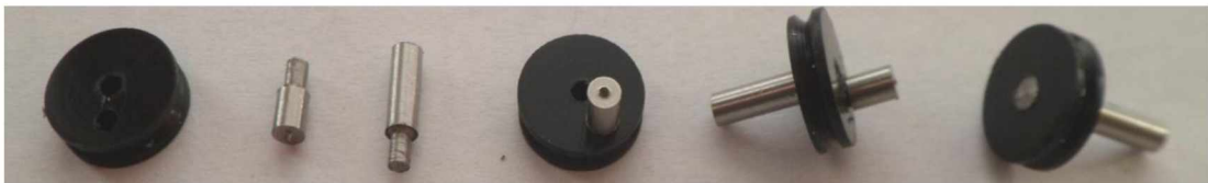
Figure 23: Additional hardware used for the pulley mechanism, showing a progression of assembly from right to left.
