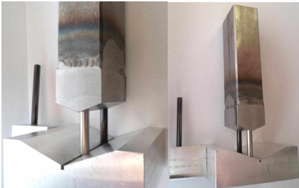
Figure 20: Bending jig used to create specified angles in the spider support compression molds.
