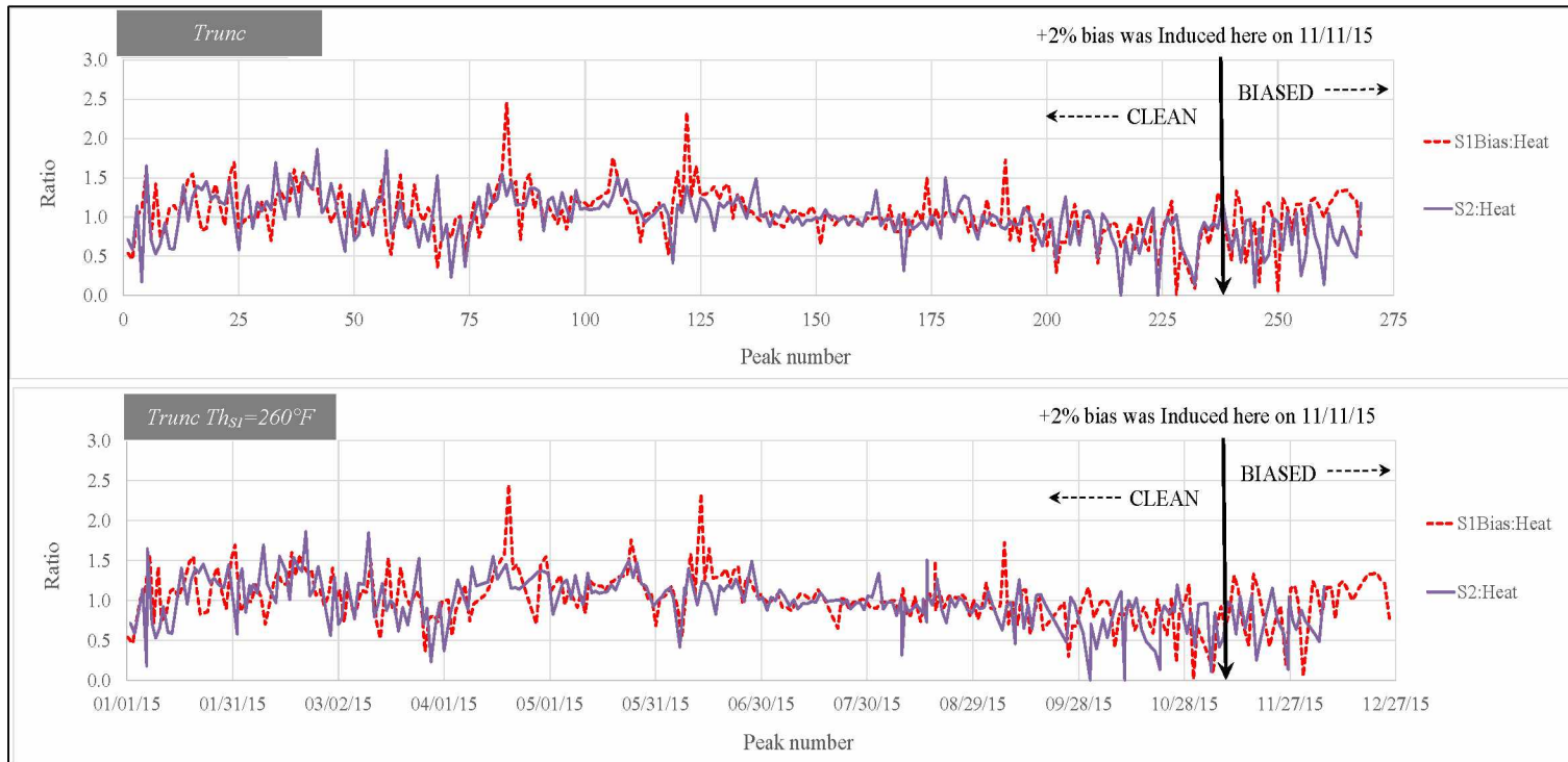
Figure 5.27: Effect of lowering the threshold to 260°F on peaks captured.
