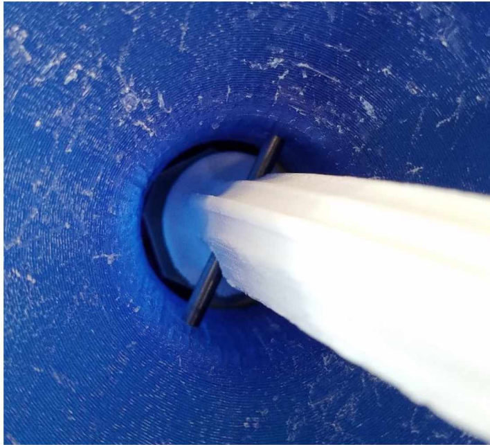
Figure 3.23: Successful test of the servo activating to push the pin through the leg and funnel
