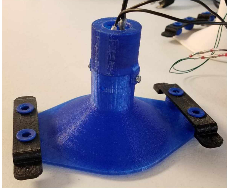
Figure 3.20: Funnel assembled with mount, vibration damping balls, and removable contact platform with contact board integrated
