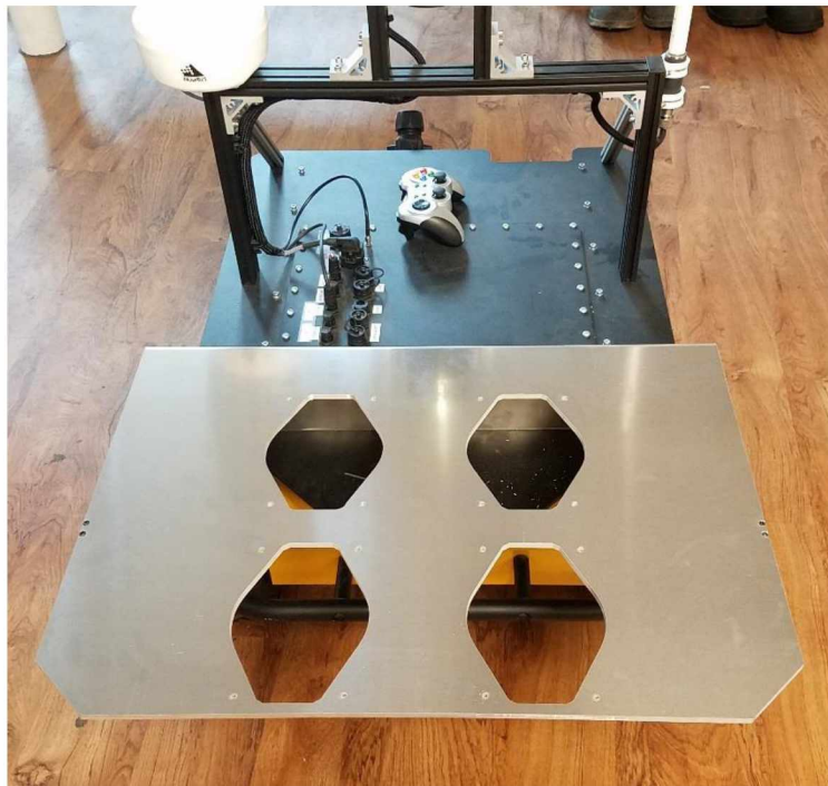
Figure 2.2: Aluminum landing pad extension created by Isaac Thompson
