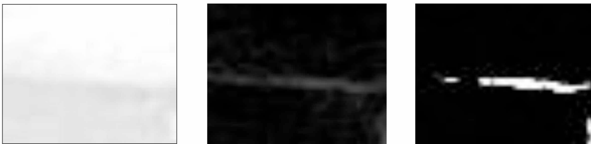
FIGURE 13. A bright image with edges (left). Sobel operator detection results (middle) and Bayesian edge detection results (right) are shown.
