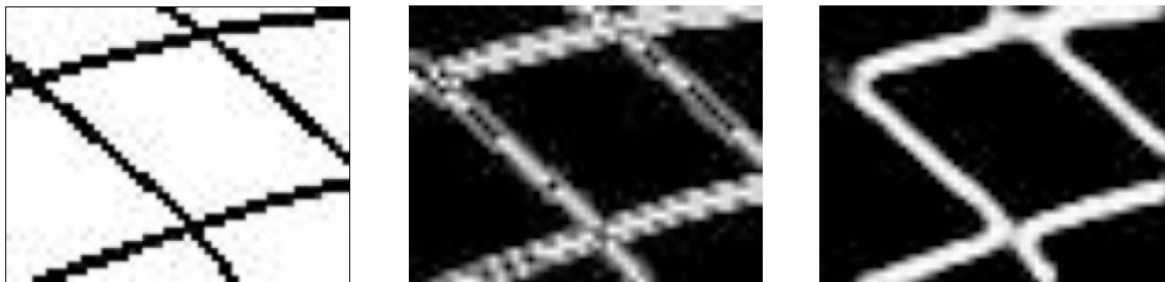
FIGURE 12. A rich photo with sharp edges (left). Sobel operator detection results (middle) and Bayesian edge detection results (right) are shown.
