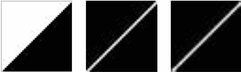
FIGURE 9. An image with a sharp edge along the diagonal (left). Sobel operator detection results (middle) and Bayesian edge detection results (right) are shown.
