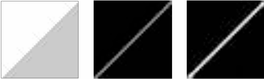
FIGURE 11. An image with a weak edge along the diagonal (left). Sobel operator detection results (middle) and Bayesian edge detection results (right) are shown.
