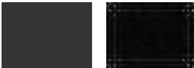
FIGURE 8. Sobel operator (left) and Bayesian method (right) edge detection results from a simulation image with smoothly varying intensity.
