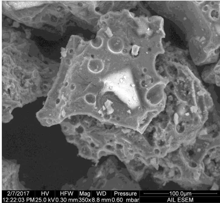
Fig. 3.6. Scanning electron image of black tephra. Scanning electron microscope image of black tephra revealing angular, vesicular fragments.
