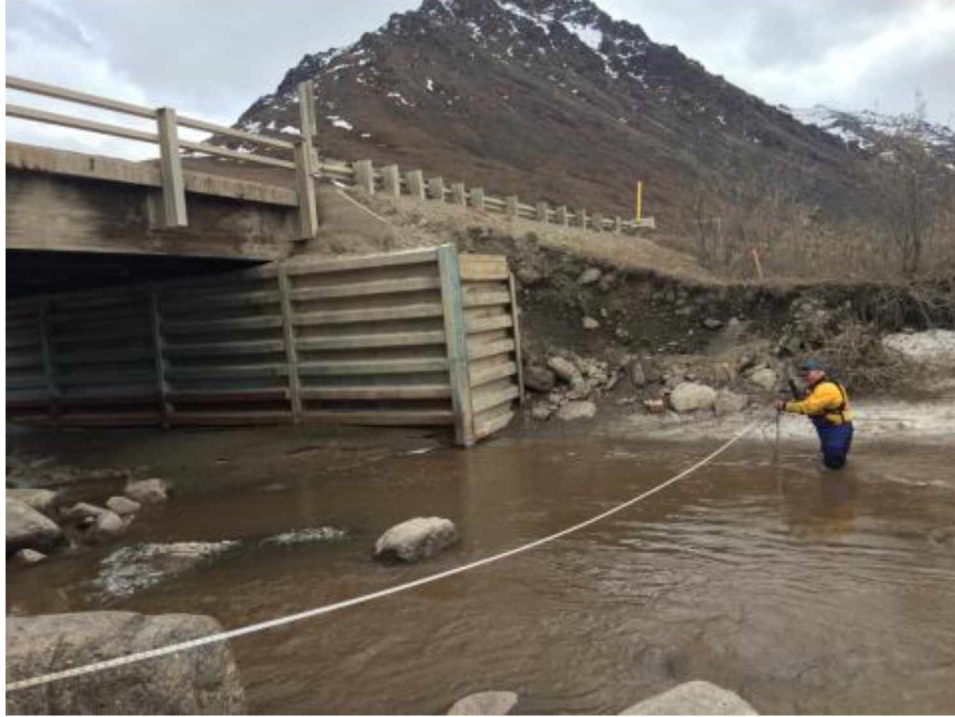
Figure 7 Manually gauging Roche Moutonnée Creek with a Price AA Current Meter in May.
