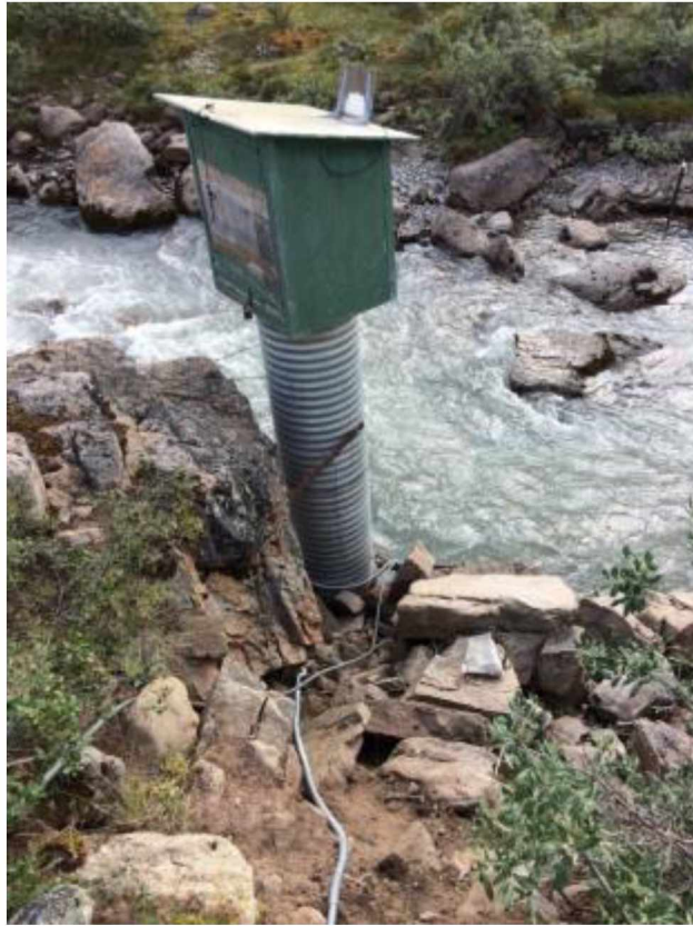
Figure 6 Roche Moutonnée Creek gauge site in July. The stilling well is USGS property. TEON staff gauge is to the right.
