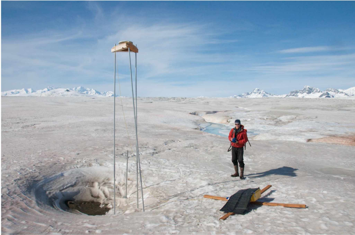
Figure 2.2. GPS Station at the End of the 2009 Melt-Season. Station CNTR is located in the ablation area where the antenna poles are drilled into ice. This photo was taken on the return trip to Yahtse Glacier, AK at the end of the 2009 melt-season.
