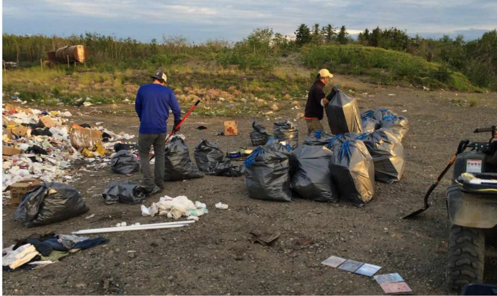
Figure 2.1. Fort Yukon Waste Characterization. Collection of Fort Yukon waste stream. Waste was sorted, separated, categorized, and weighed.
