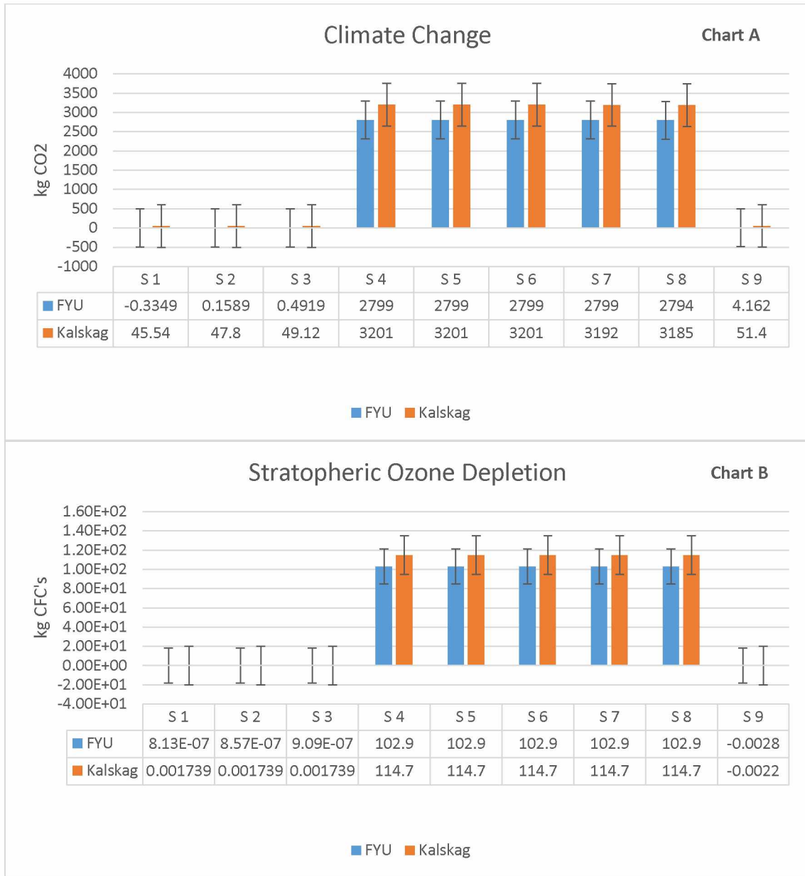
Figure 3.5. Air Impact Categories. Scenario 1-9. Chart A: climate change/global warming measured by kg of CO 2 released per kg of waste. Chart B: stratospheric ozone depletion as kg of CFC's released per kg of waste. Chart C: particulate matter measured as kg PM 2.5 released per kg of waste. Chart D: photochemical ozone formation measured by 1 kg of NO x and VOC per kg of waste and .0456 kg CO per kg of waste. The intervals represent the confidence interval of standard errors. FYU=Fort Yukon
