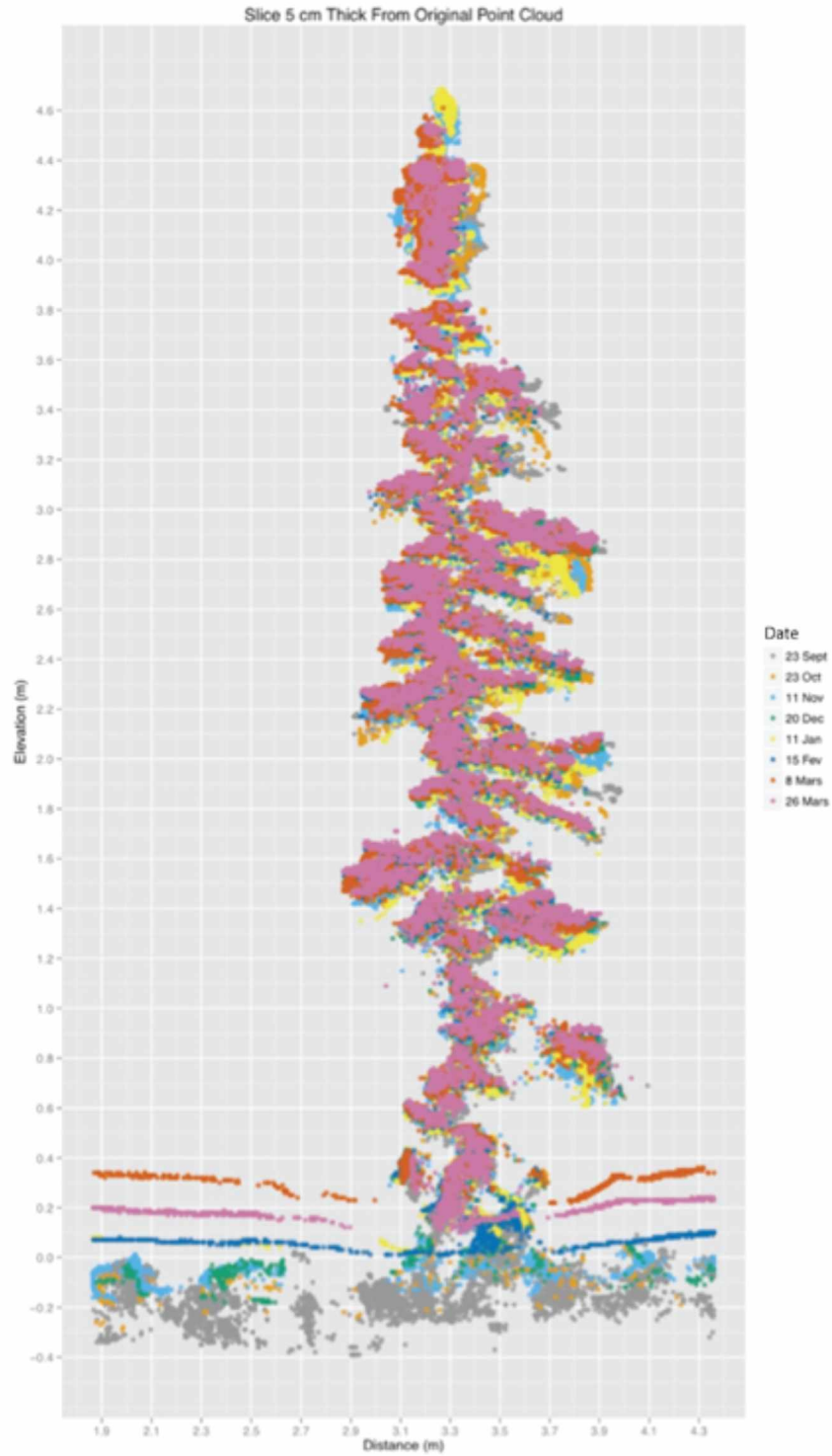
Figure 4.8: A 5 cm thick vertical slice of the season 2011-2012 lidar point clouds. Colors indicate the date of scanning. The spruce tree is marked in Figure 4.1.
