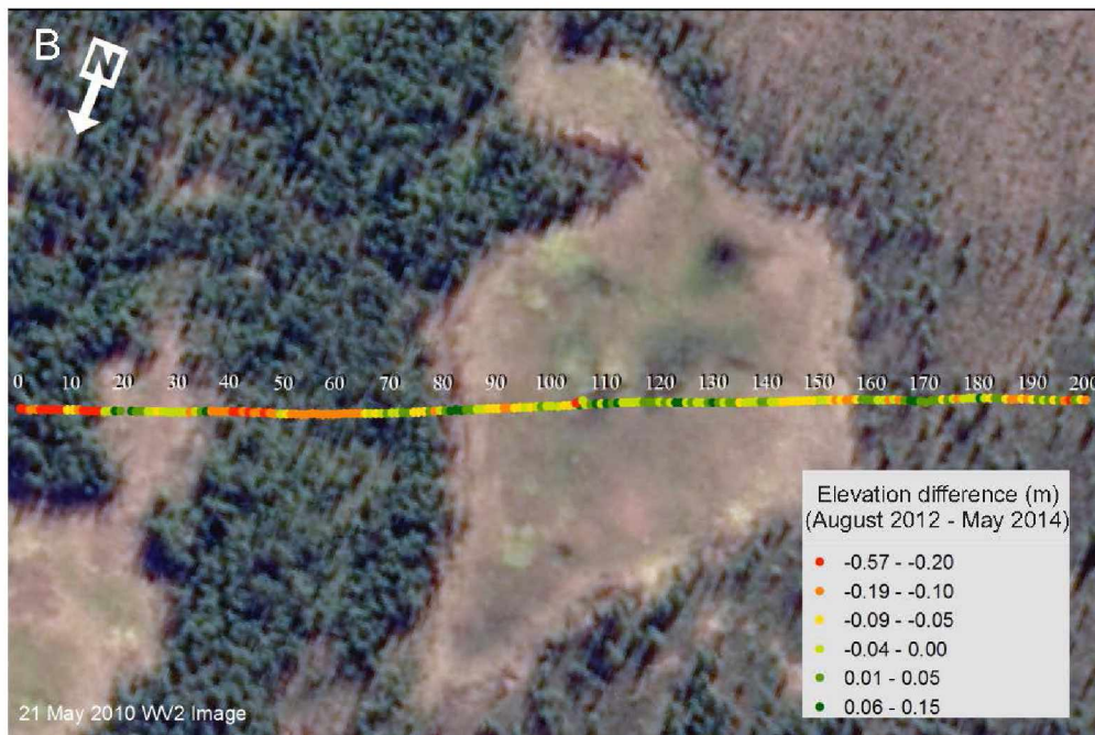
Figure 1.7. Transect through burned black spruce forest and collapse-scar bogs in the 2010 fire scar. (a) A cross-section of a portion of the transect depicts the elevations (m) of the ground surface, surface water, permafrost table, and maximum observed depths of unfrozen ground over time. Measurements for 2013 from transect meters 0 to 25 were excluded due to dGPS inaccuracy. (b) A bird's-eye view of the transect, overlain on prefire imagery (WorldView2, 21 May 2010), shows an independent comparison of surface elevation over time using ground-based dGPS (August 2012) and airborne LiDAR (May 2014).
