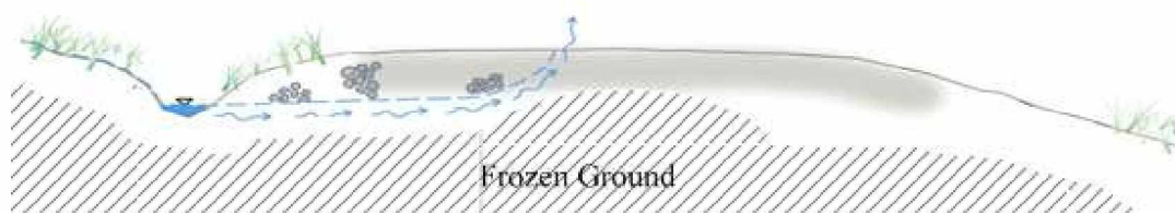
Figure 1.1 Pressurized Ground Water Flow in Spring
