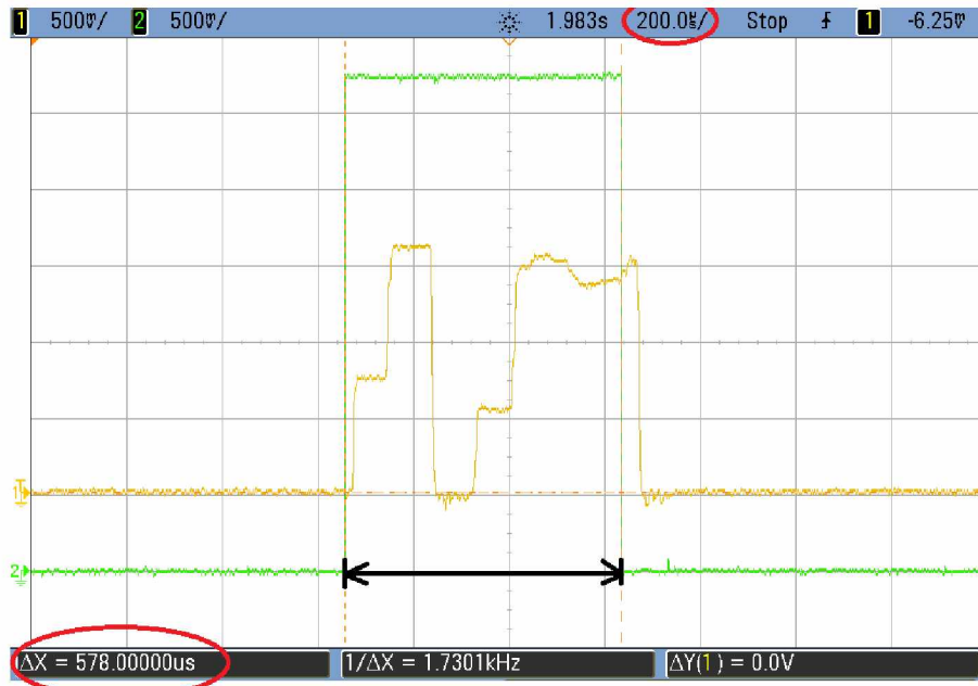
Figure 24: TX-RX transaction's duration of a 3-bytes payload packet (578 \mu s )
