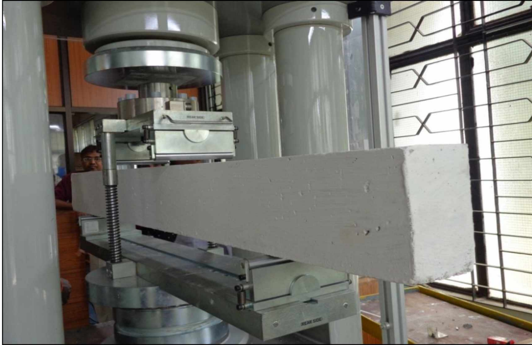
Figure 4.11: Beam when Placed in the Test Setup (Gopinath et al. 2014)
