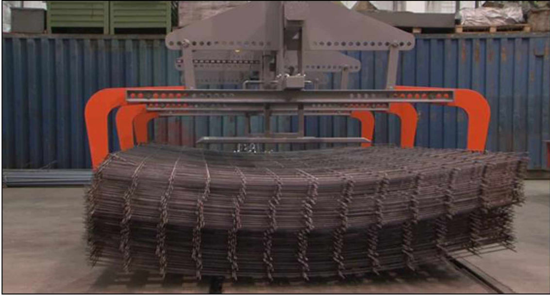
Figure 1.8: Crane Handling of Welded Wire Reinforcement Bundle (Schnell 2015)
