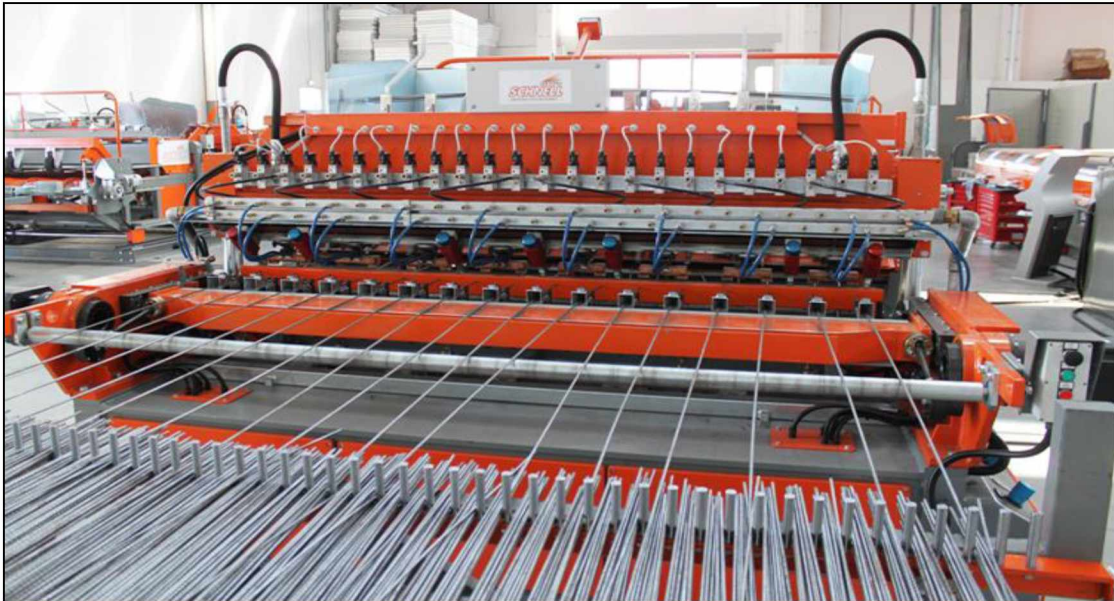
Figure 1.6: Longitudinal Wire Fed into Automated Welding Machine (Schnell 2015)
