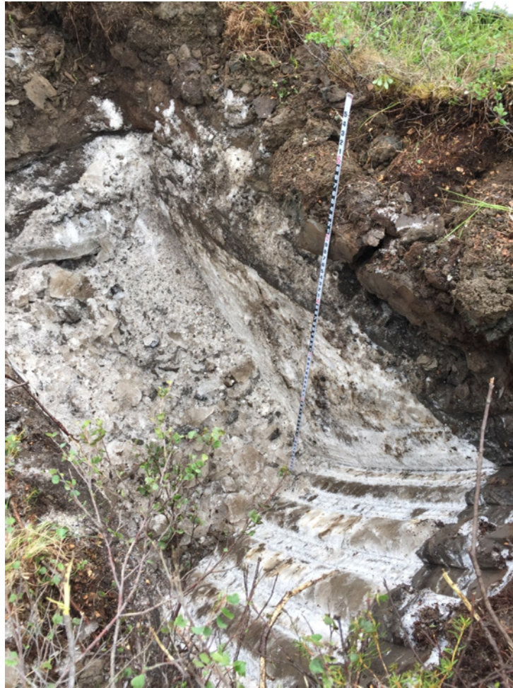
Figure 4: Test Pit at Potential Landfill Site in Buckland, Alaska.
