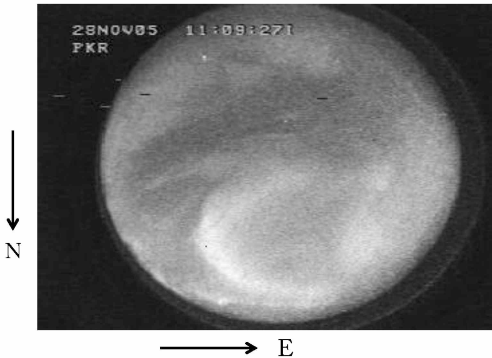
Fig 3.12. Example black and white all sky camera image. This image represents a traditional black and white all sky image which may be utilized to calculate total auroral luminosity.
