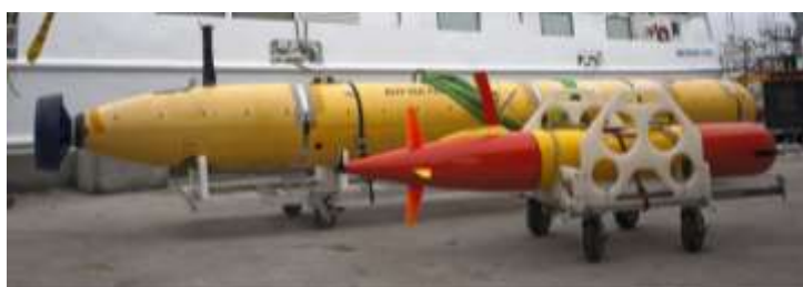
Figure 8. The Tethys LRAUV (foreground) is much smaller than the Dorado platform providing a cost-effective solution for multivehicle operations.
