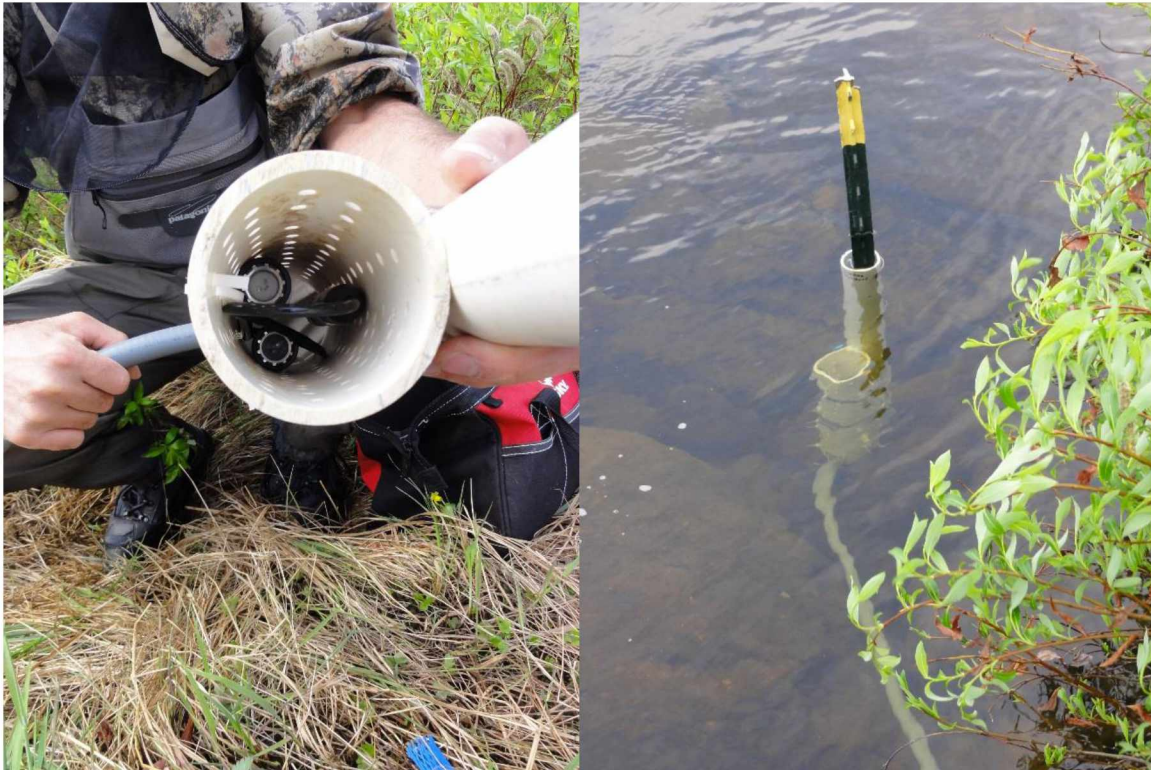
Figure 3.2 Sensor installation on the Kuparuk River.
