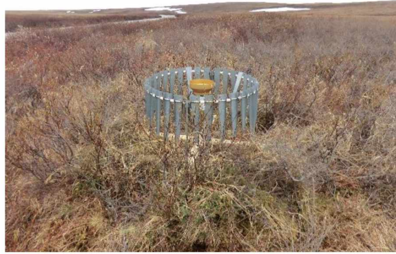
Figure 3.1 A TE525MM tipping bucket surrounded by a metal alter shield.
