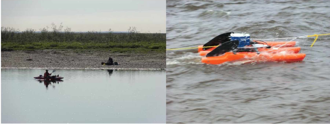
Figure 3.3 The two methods of taking a measurement with the StreamPro.
