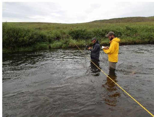
Figure 3.4 Velocity measurement using the Flow Tracker. Levi Overbeck (left) and Tyler King (right) perform a velocity measurement using the Flow Tracker on the Kuparuk River.
