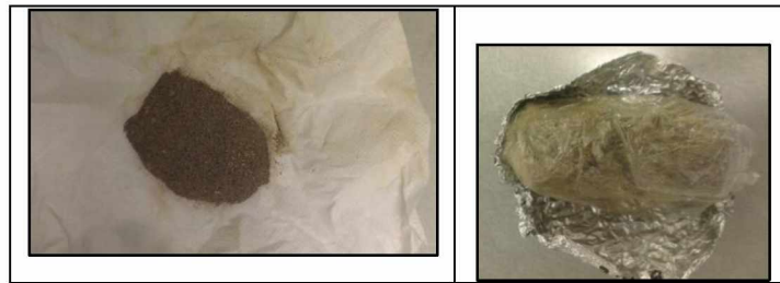
Figure 4.5 Core Sample Disintegrated into Sand after Dean-Stark Experiment and Already Broken Core Samples (in transportation)
