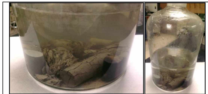
Figure 4.6 Pictures of Damaged Core Samples after Saturating in High Salinity Brine
