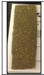
Figure 4.14 Substrate Prepared by Directly Sprinkling Clay on the Slide (Glauconite)
