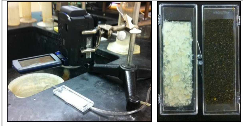
Figure 4.12 Video Camera Setup and Substrates of Kaolinite and Glauconite clay
