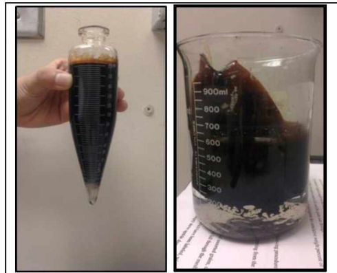
Figure 4.3 Picture of Filtered and Centrifuged Oil after Addition of Emulsion Breaker, which shows the Removed Water (Sample from Well 2)
