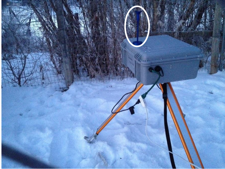
Figure 2.10. The instrument setup for the DustTrak during the Sled Dog Air Contaminant campaign. The inlet is outlined by the white circle.
