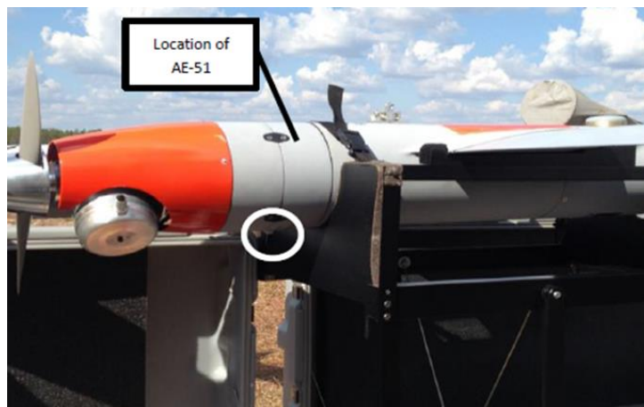
Figure 3.4. Boeing ScanEagle with AE-51 microAethalometer onboard. The white circle shows the inlet tube of the microAeth sticking out of the bottom of the aircraft.
