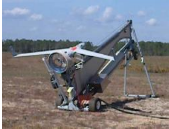
Figure 2.11. Boeing ScanEagle ready for takeoff on a Mark 4 launcher.
