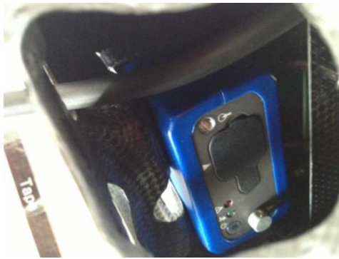
Figure 3.3. Image showing the placement of the AE-51 microAethalometer in the fuselage of the Boeing ScanEagle.
