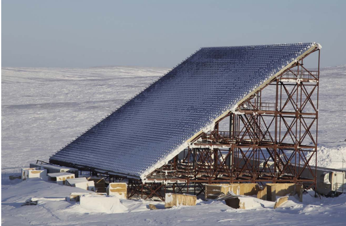
Figure 5.2: Northward looking UHF phased array radar at Resolute Bay, on Cornwallis Island, Canada.
