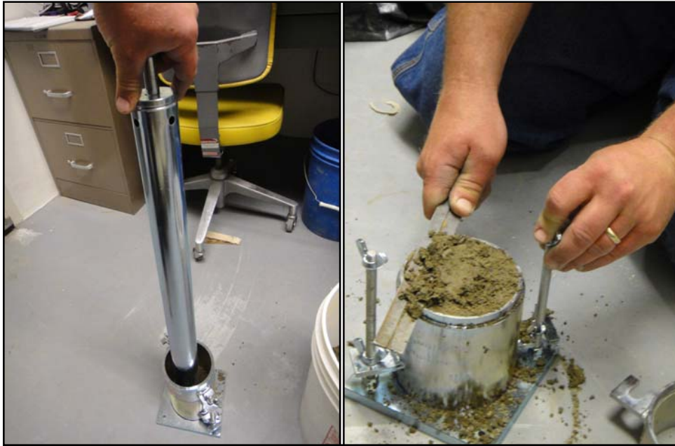
Figure 3.9: Equipment used during moisture-density relationship analysis. Modified compaction hammer and 4 inch Proctor mold (left). Preparation of sample within 4 inch Proctor mold (right).
