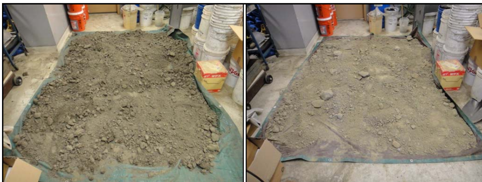
Figure 3.1: Photographs of the air-dried soils. Studied silt (left), and studied silty gravel (right).
