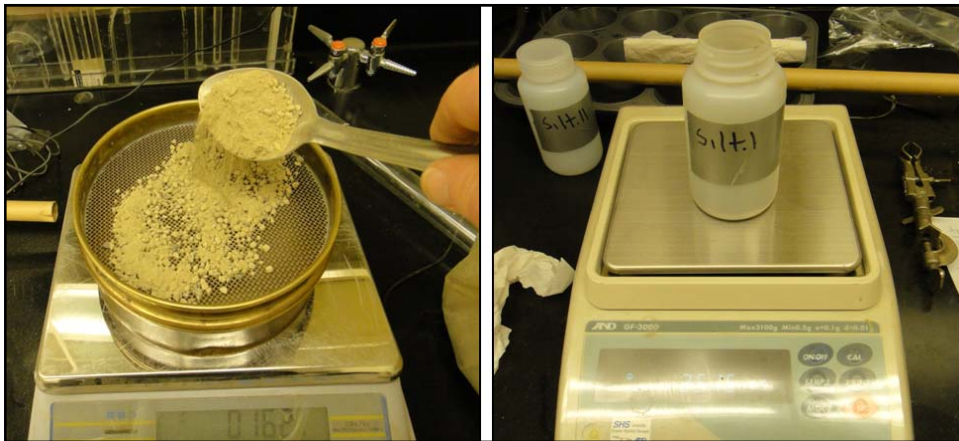
Figure 3.5: Preparing sample of soil for pH measurements. Sieving a 350 gram sample (left) and weighing a 25 gram sample (right).
