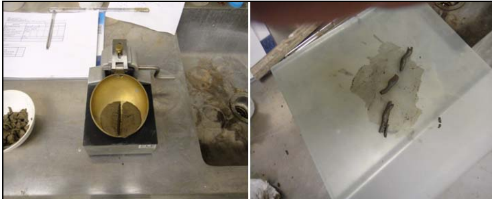
Figure 3.4: Conducting Atterberg limits testing on studied soil. Sample of soil within liquid limit device (left) and on plastic limit plate (right).
