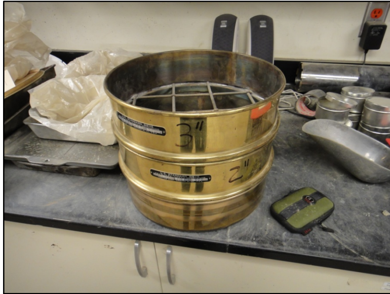
Figure 3.2: Round 12-inch diameter sieves used during gradation analysis of the silty gravel.
