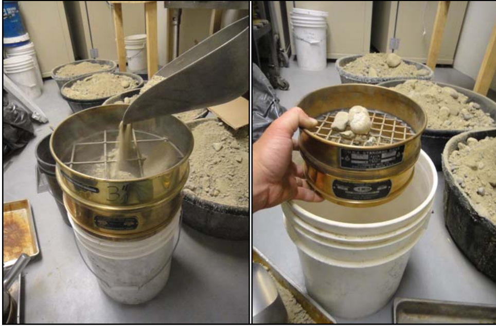
Figure 3.8: Preparation of the silty gravel for moisture-density and 5,000-pound analyses. Obtaining 3 inch-minus/ \frac{3}{4} inch-plus material (left) and obtaining \frac{3}{4} inch-minus/No. 4-plus material (right).
