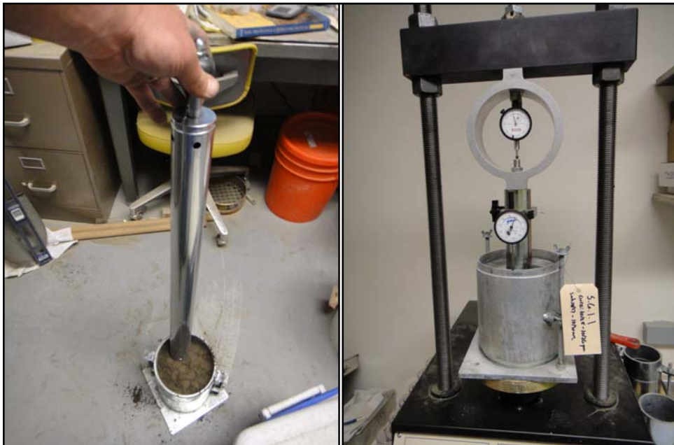
Figure 3.10: Equipment used to measure CBR of the silt. Sample of silt compacted within a 6 inch CBR mold (left). Molded sample within CBR press (right).
