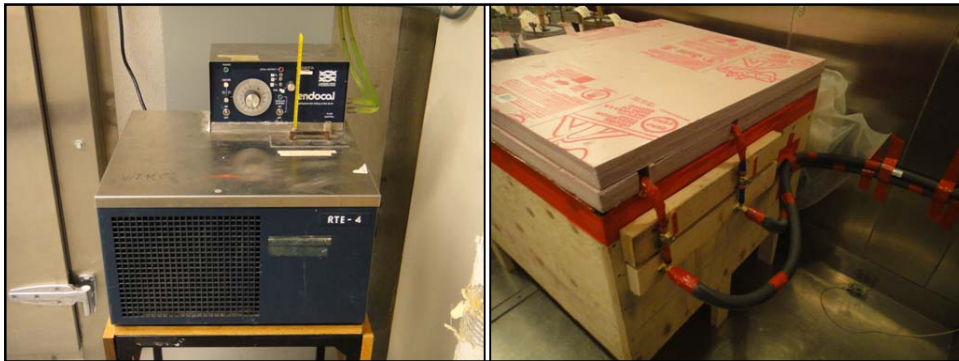
Figure 3.12: Equipment used during the freeze tests. Endocal circulating heater (left). Plumbed PEX lines extending into freezing apparatus (right).
