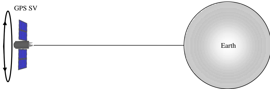
Figure 11: SV Yaw Attitude Changes to Optimize Solar Panel Orientation in Orbit
