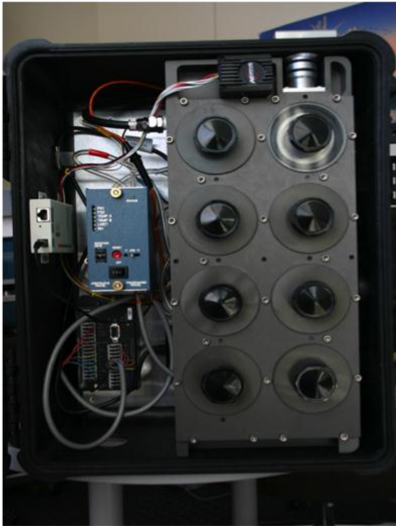
Figure 3-5. Photograph of a Davis rotating drum unit for monitoring (DRUM) aerosol impactor.
