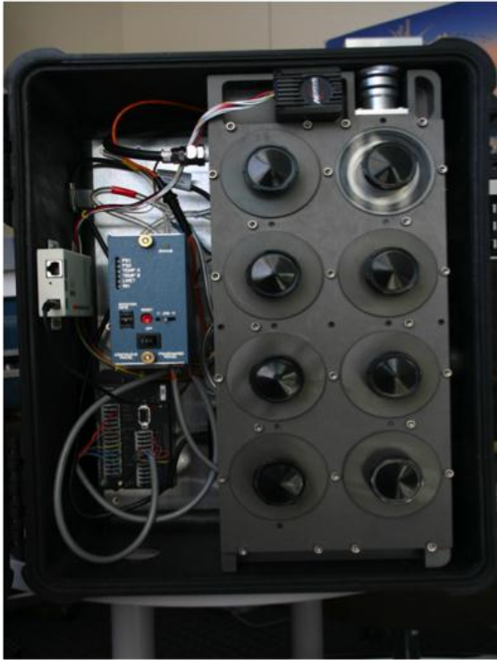
Figure 2-4. Photograph of a Davis rotating drum unit for monitoring (DRUM) aerosol impactor.
