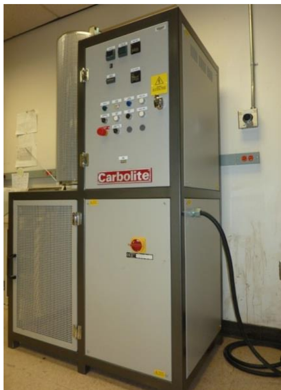
Figure 43: Customized Thermal Cycling Furnace Designed by Carbolite Inc.
