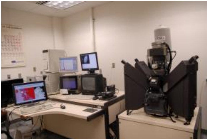
Figure 41: CAMECA SX-50 Electron Microprobe with EDAX EDS System
