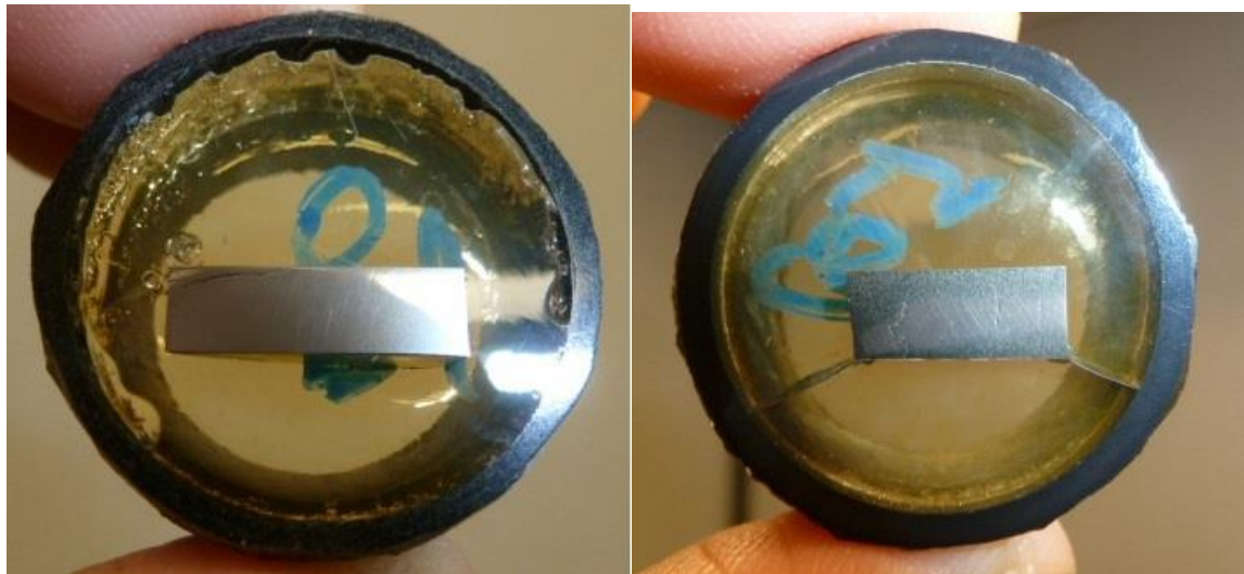
(c) Cross-section of HTM (As-Received) (d) Cross-section of HTM (500 Thermal Cycles)
