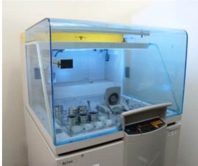
Figure 40: Panalytical Axios Four Kilowatt Wavelength Dispersive Spectrometer (WDS) X-ray Florescence (XRF)
