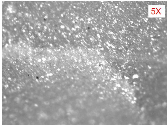
Alumina 99 wt% (CoorsTek) - Fracture Surface
