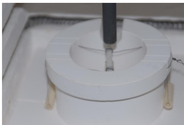
(b) Specimen Setup for Young's Modulus Measurement at High Temperature
