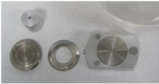
(a) Sample holder for powder
