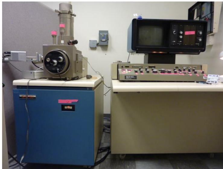
Figure 34: Scanning Electron Microscope (SEM) ISI-SR-50 Automated with iXRF Software/Hardware and EDS Detector
