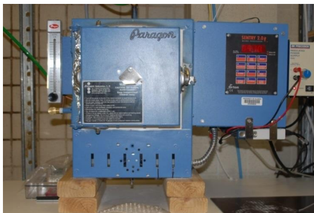
(a) System Setup for Young's Modulus Measurement at High Temperature
