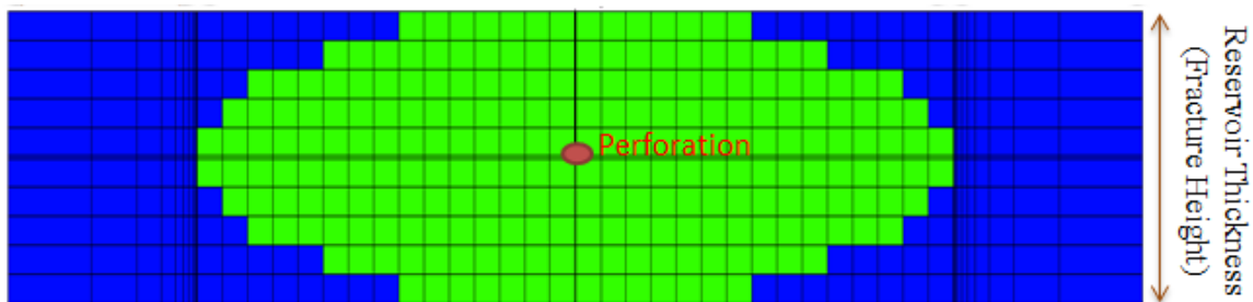
Figure 21: Side view of simulation model at fracture plane; matrix blocks and hydraulic fracture blocks are represented by blue and green colors, respectively.
