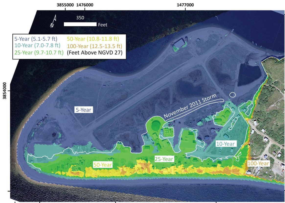
Figure 4.15—Flooding projections on the Golovin spit from numerical modeling and measured storm events, projected in NAD83 State Plane, Alaska 7 (in feet), datum NGVD 27 (feet). Base map is an aerial photograph flown in June 2004, provided by the Alaska DCCED (all elevations and spatial references were provided in feet for the use of these values by the community of Golovin in the future).
