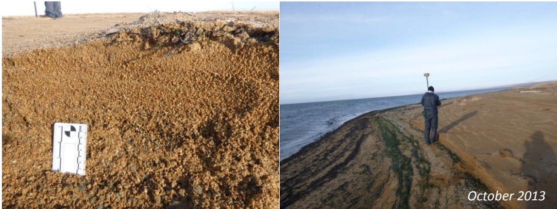
Figure 2.9—Intertidal scarp formed during Oct. 2013 storm at Profile 6 on end of spit (measured by Alexander Gould).
