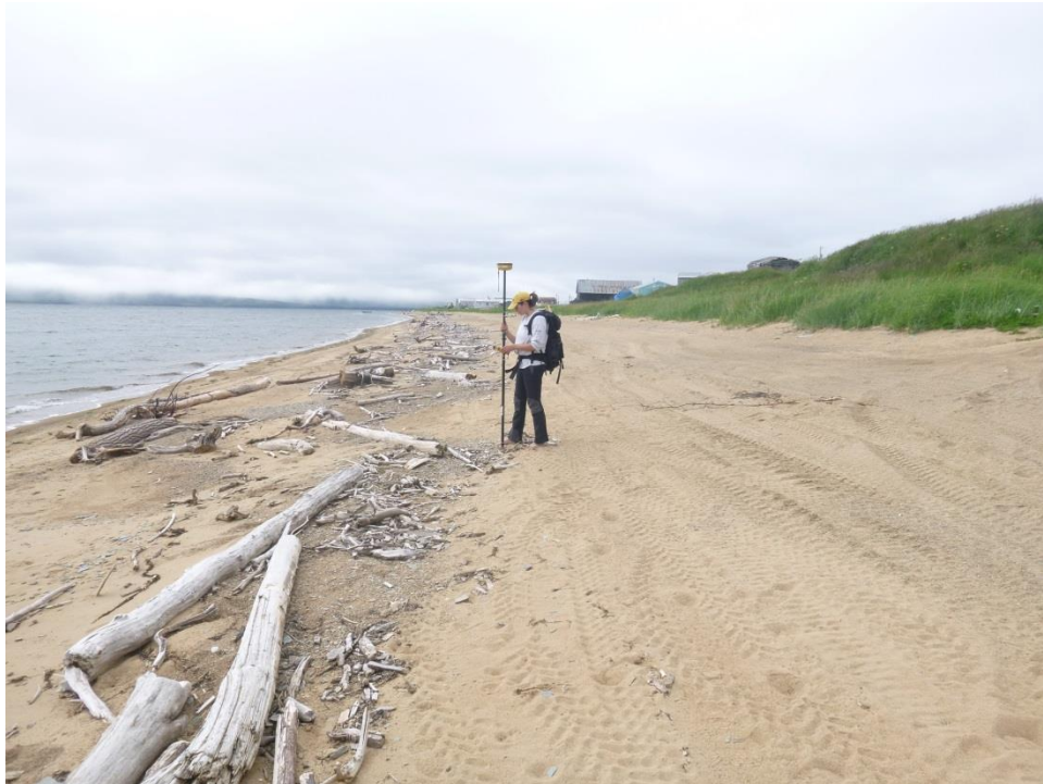
Figure 2.4—Example of cross-shore beach survey at inland extent of woody-wave-carried debris (Kimber Tweet holding the GPS rod).
