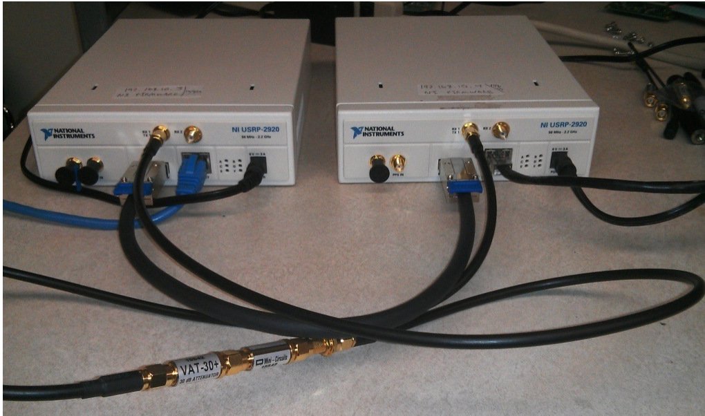
Figure 4.1. Lab Setup - 2 NI USRP 2920
