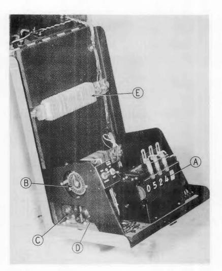
Figure 5 - Control Box of Synchronous Model
