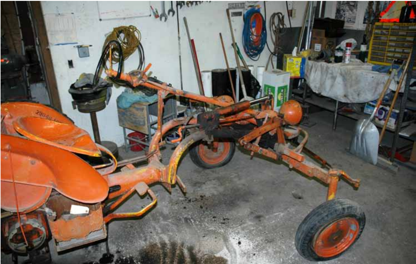
Photo B: The Chalmers 'G' being stripped down (seeder removed). Below: engine housing.
