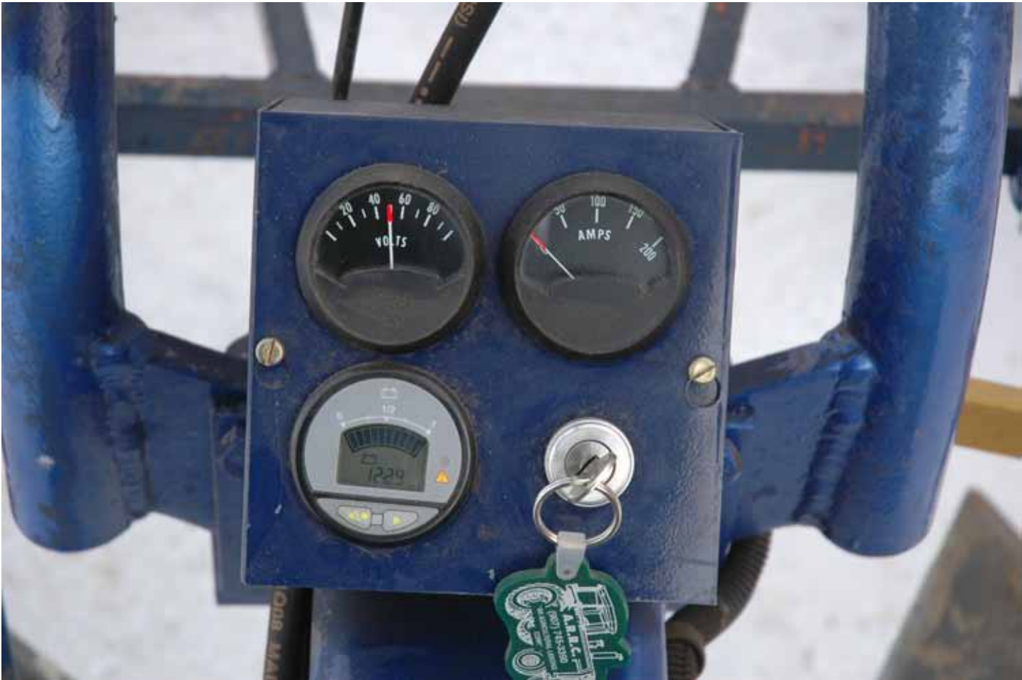
Photo F: Instrument panel. From bottom left clockwise: engine hour meter, voltage meter, amperage meter, on/off switch with safety shutoff on key removal.
