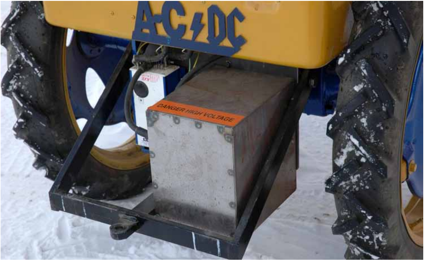
Photo G: electric drive controller.
