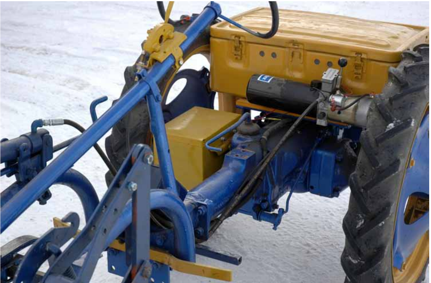
Photo I: Hydraulic pump and toolbar of the refurbished tractor.
