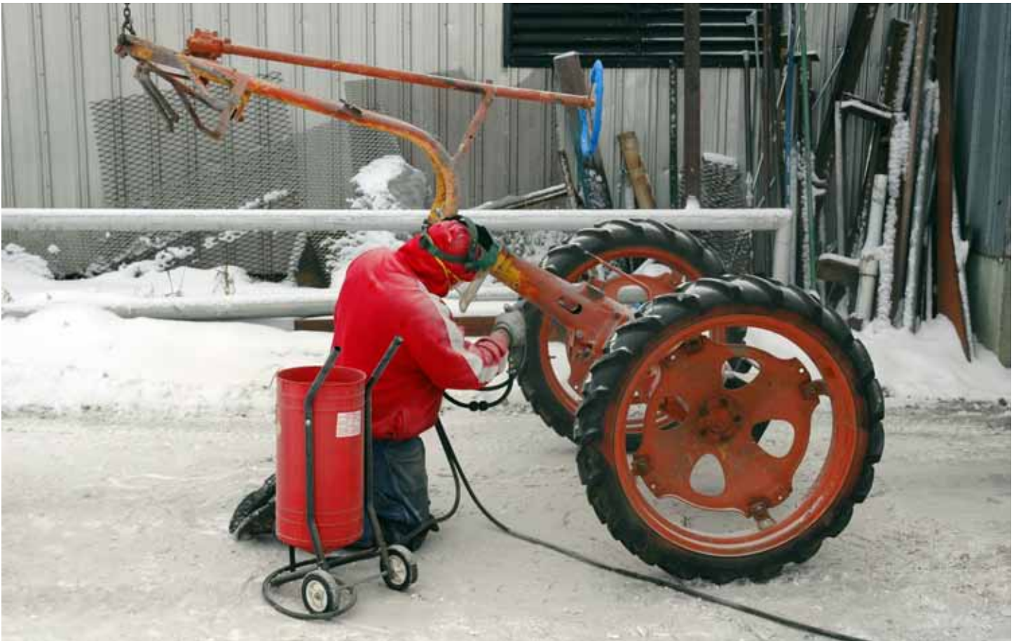
Above, sandblasting the tractor frame and below, painting it in the shop.
