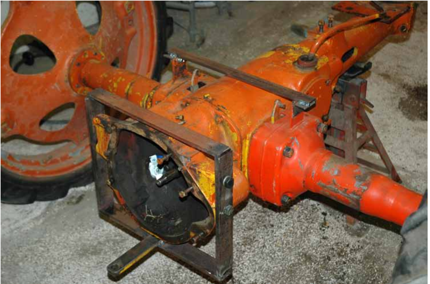
Photo C: More views of the disassembly. Above: engine housing. Below: housing frame.
