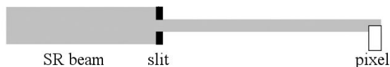
Figure 1. Set-up for the implementation of the edge illumination method with synchrotron radiation: the beam coming from the left is shaped with a slit which is aligned with the edge of a detector pixel.
