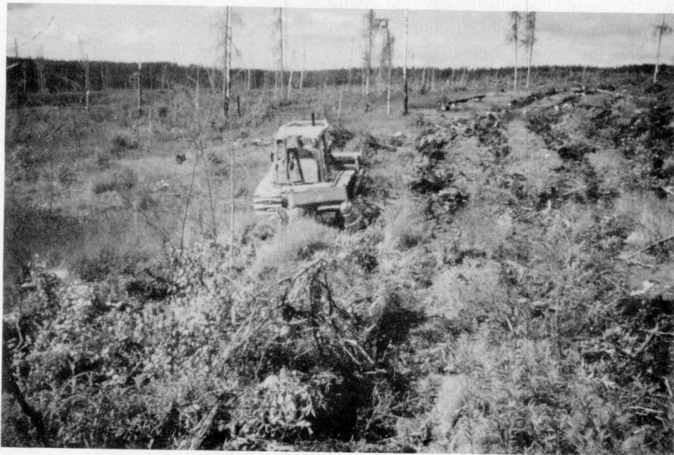
Figure 5. Photo showing the D-6 crawler and the spacing of the furrows obtained.
