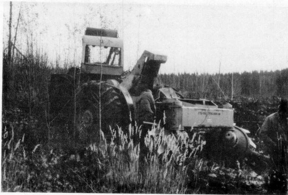
Figure 4. Photo showing the TTS-35 being towed behind the Clark 668 rubber-tired skidder used by Contractor #3.
